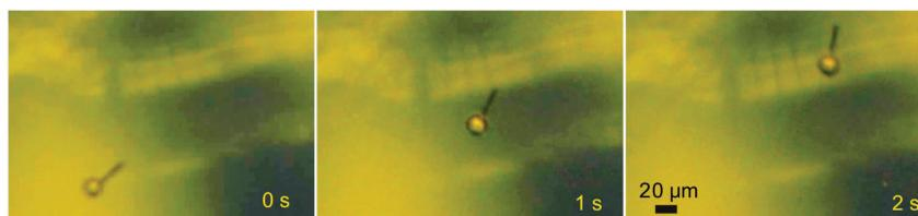
**Figure 5** Time-lapse images of a moving nanoporous microengine (with 150-nm nanopores on the wall) at a low fuel concentration of 0.2%.
