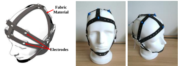
Fig 8. The structure and prototype of the smart hat
