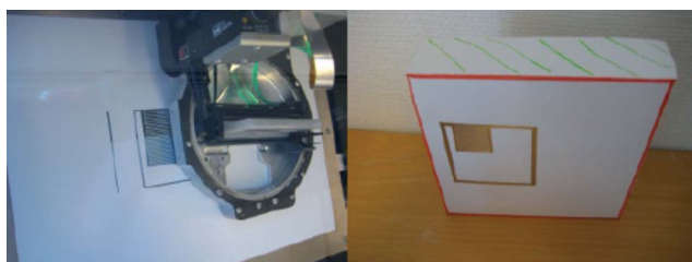
Fig. 6 (left) Inkjet printing process of the proposed RFID tag; (right) RFID tag directly printed on packaging paper.
