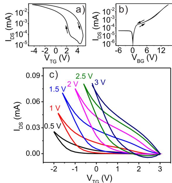
FIG. 2. (a) Transfer curve  $I_{\text{DS}}-V_{\text{TG}}$  with constant  $V_{\text{DS}} = 1$  V when the gate voltage was applied on TG. (b) Transfer curve  $I_{\text{DS}}-V_{\text{BG}}$  with constant  $V_{\text{DS}} = 1$  V when the gate voltage was applied on the bulk silicon (BG). (c) Transfer curves  $I_{\text{DS}}-V_{\text{TG}}$  with different  $V_{\text{DS}}$ .
