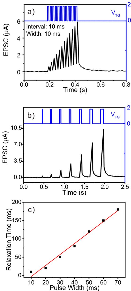
FIG. 4. (a) EPSC responses of the device to stimulus train with a 12 gate spikes (2.0 V, 10 ms). The  $V_{DS}$  is fixed at 1 V. (b) The width of the presynapse spike on the gate electrode was changed from 10 to 70 ms. (c) EPSC relaxation time as a function of input pulse width. The black squares are experimental results. The red line is the relaxation time behavior fitted by the linear function.
