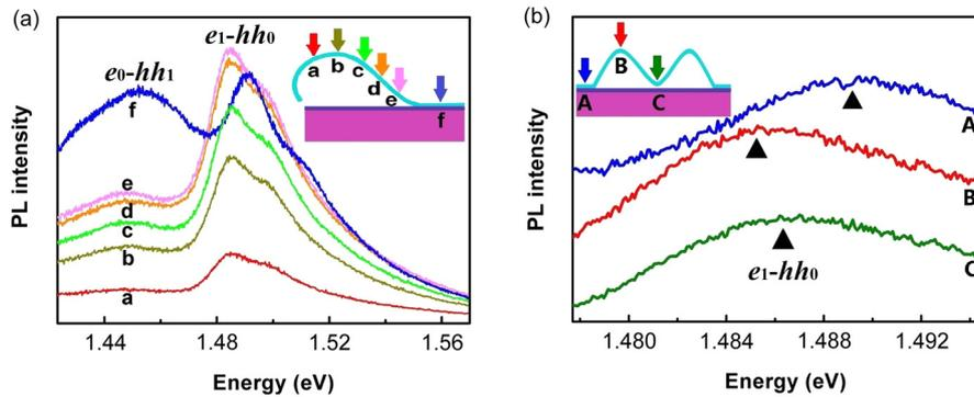
**Fig. 3.** (a) PL spectra of a rolled-down nanomembrane. (b) Enlarged view of  $e_1$ - $hh_0$  transitions of PL spectra for a wrinkled membrane. The colors of the plots correspond to the laser position marked by arrows with the same color (inset). Blue color corresponds to the result from the flat nanomembrane.
