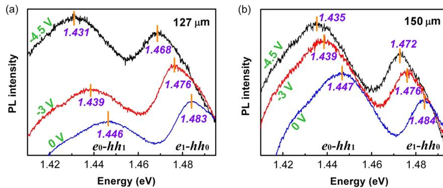
**Fig. 4.** PL spectra of rolled-up nanomembranes with diameters of 127  $\mu\text{m}$  (a) and 150  $\mu\text{m}$  (b) at room temperature. The excitation wavelength is 540 nm. Bias voltages of 0,  $-3$ , and  $-4.5$  V were applied to the samples and the energies of  $e_0$ - $hh_1$  and  $e_1$ - $hh_0$  peaks are labeled.
