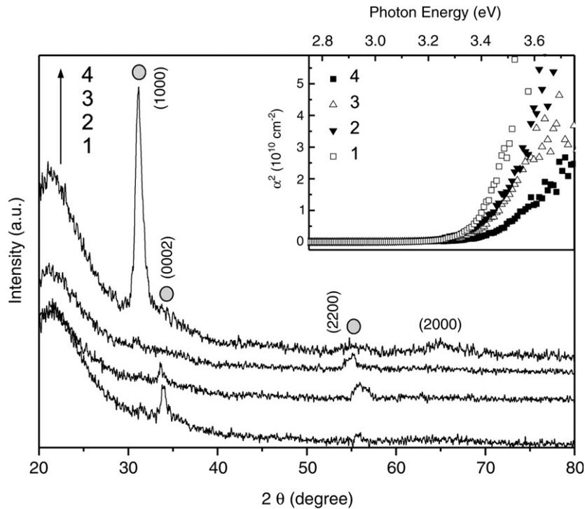
Fig. 2. XRD patterns acquired from ZnO films deposited on fused quartz. No. 4 and No. 1 were fabricated using a similar as samples A and B, respectively. No. 2 was produced using a DC sample bias  $-100$  V and No. 3 was synthesized using a mixture of  $O_2$  and  $N_2$  at a DC bias of  $-300$  V.
