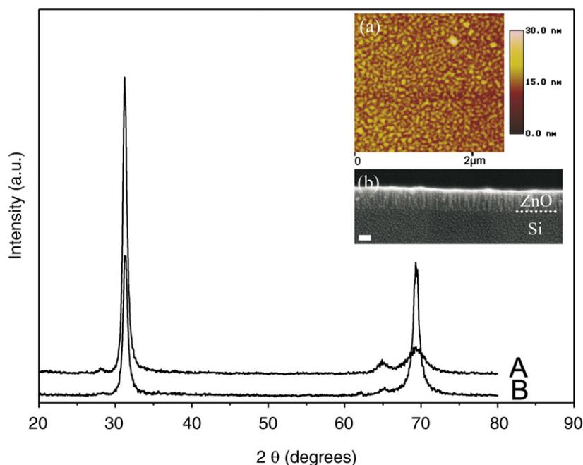
Fig. 1. X-ray diffraction patterns obtained from ZnO films deposited on Si at two different distances (A: 10 cm and B: 20 cm). Shown in inset (a) is the surface AFM micrograph and inset (b) the cross-sectional SEM micrograph [the scale bar is 100 nm] of sample B.
