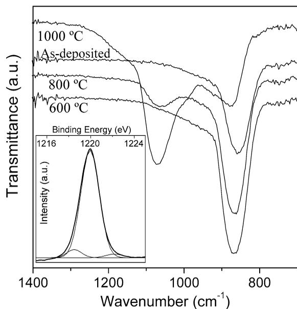
Fig. 2. FTIR spectra of Ge oxide film deposited at 200 °C and the samples subsequently annealed at 600–1000 °C in N<sub>2</sub> for 30 minutes; the inset shows the XPS results of Ge oxide film deposited at 200 °C and subsequently annealed at 800 °C in N<sub>2</sub> for 30 minutes.
