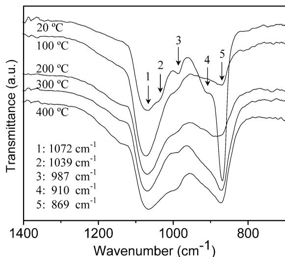
Fig. 4. FTIR spectra of Ge oxide film deposited at different substrate temperature [from room temperature (20 °C) to 400 °C] and subsequently annealed at 1000 °C in N<sub>2</sub> for 30 minutes.
