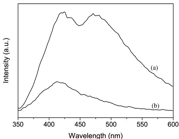
Fig. 3. PL spectra of Ge oxide film deposited (a) at 200 °C under oxygen pressure of  $\sim 6.5$  Pa and annealed at 600 °C, (b) at room temperature under oxygen pressure of  $\sim 100$  Pa and annealed at 800 °C. (Their intensities are strongest in their corresponding group samples.)
