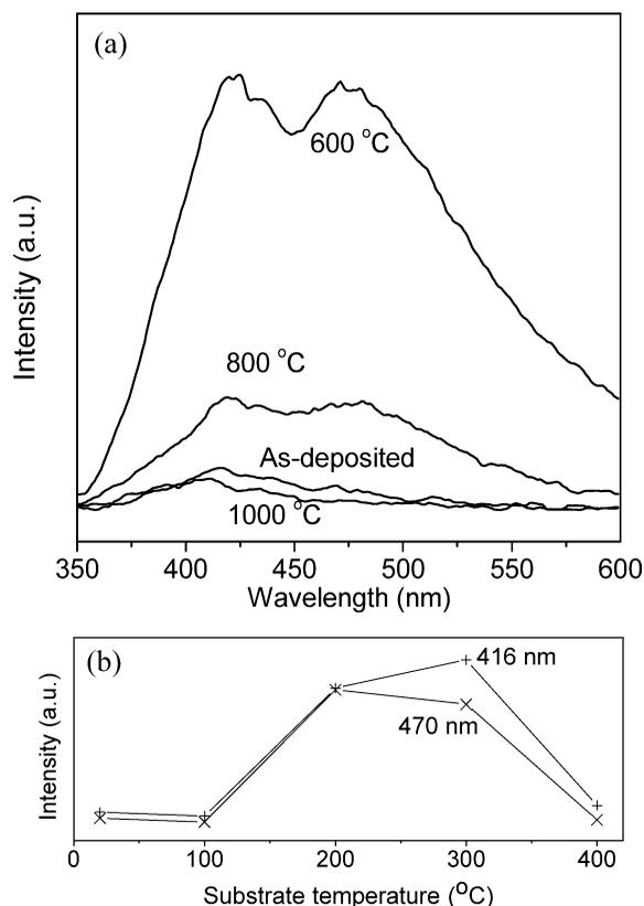
Fig. 1. (a) PL spectra of as-deposited sample deposited at  $200^\circ\text{C}$  and the samples subsequently annealed at  $600$ – $1000^\circ\text{C}$  in  $\text{N}_2$  for 30 minutes; (b) dependence of the PL (416 and 470 nm) maximal intensity on substrate temperature.
