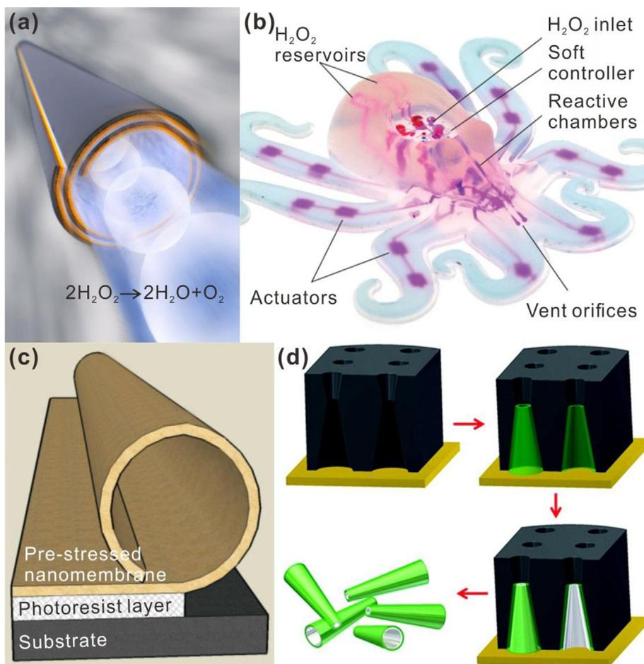
**Fig. 1.** (Color online) (a) Scheme depicting self-propelled tubular micro/nanoengines [2]. (b) Optical images of a fully soft, autonomous octobot powered by hydrogen peroxide decomposition [3]. (c) Scheme illustrating the rolled-up nanotechnology to fabricate tubular microengines [2]. (d) Scheme of bilayer tubular microengines using polycarbonate membranes [4].
