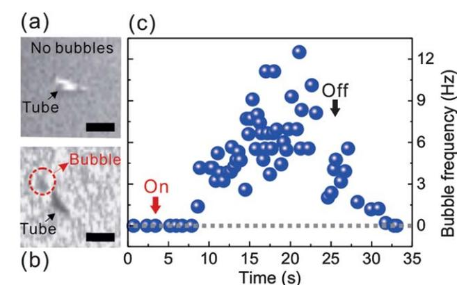
**Fig. 3** (a) Optical image showing an inactive microtubular engine with no bubbles generated under a low concentration of fuel. Once illuminated under a laser, the engine starts to generate bubbles. Shown in (b) is the optical image with laser on for 4.5 s. (c) The graph presents the dependence of bubble generation frequency on the irradiation time of the laser, in which the “On” and “Off” refers to laser on and off. All scale bars: 50  $\mu\text{m}$ .
