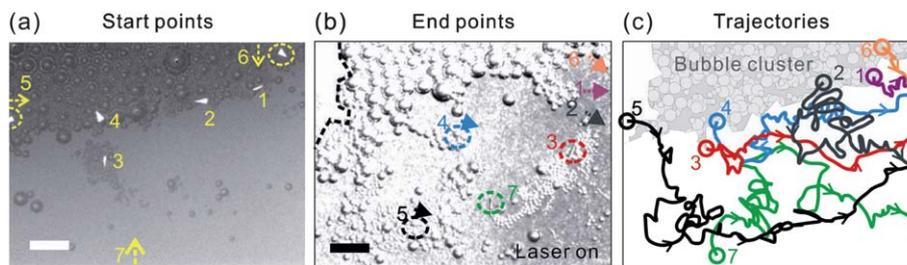
**Fig. 2** (a) The image shows the tubular microengines (labelled as #1–7) initially berthed at the borders of bubble clusters without laser irradiation. During the laser irradiation, these microengines actively moved away from the bubble clusters in different trajectories, in which the final snap is shown in (b) and trajectories of the engines are recorded in (c). All scale bars: 200  $\mu\text{m}$ .
